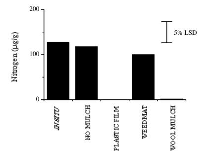
Fig. 17. The potential loss of nitrate nitrogen by leaching from the top 5cm of soil under different mulch treatments (*In situ*, no mulch, plastic film, weedmat and wool mulch). Leaching was from soil cores 3cm diameter x 5 cm high. The least significant difference at P $\cdot$ 0.05 is indicated
