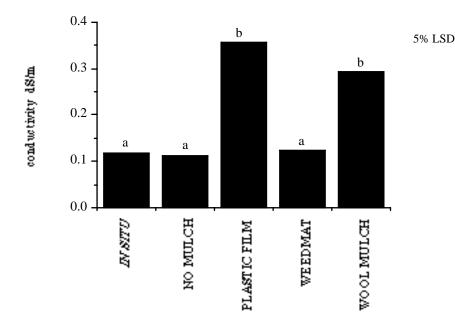
Fig. 18. Soil conductivity (dS/m) in the nitrogen incubation tubes following a 94 day incubation under the five mulches (*In situ*, no mulch, plastic film, weedmat and wool mulch). Letters indicate levels of significance at P•0.05.
