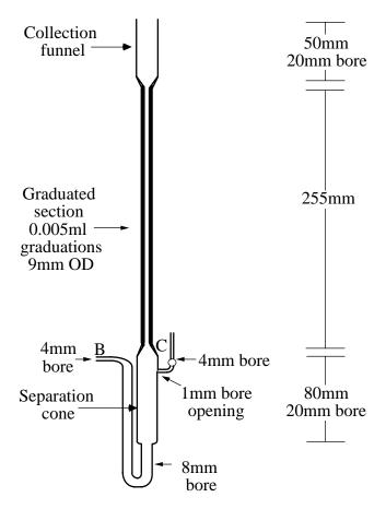
Figure 3. Semi-micro Separator
