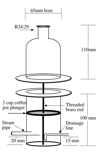
Figure 1. The Steam and Steam and Water Still Pot
