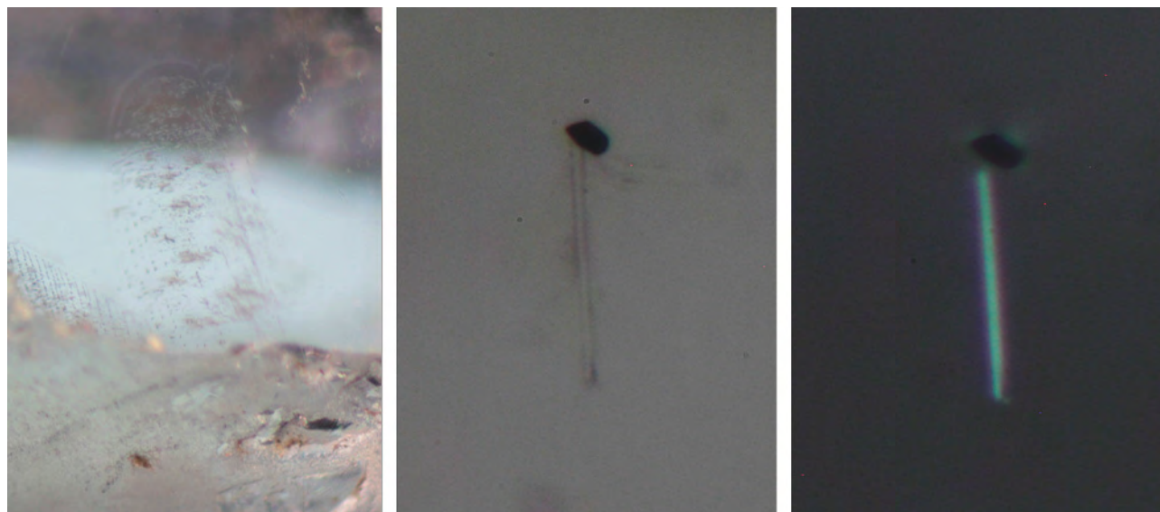
Figure 5. Blue spinels (here, GREBLU3) often show healed fractures (fingerprints, left), and some samples contain irregular opaque black crystals associated with elongated tubes (center and right). Photos by Boris Chauviré; field of view 1 mm (under daylight equivalent light on the left, plane-polarized light in the center, and cross-polarized light on the right).
