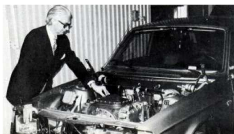
Figure 2: Prof. Kronogård with his three-shaft AGT installed in a Volvo test automobile [2].
