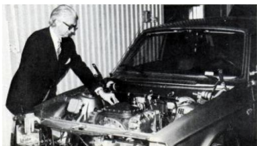
Figure 2: Prof. Kronogård with his three-stage AGT installed in a Volvo test automobile [2].
