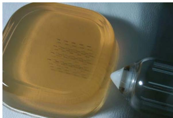
Figure 4. Experiment with stainless seeds inserted in mock-up tissue
