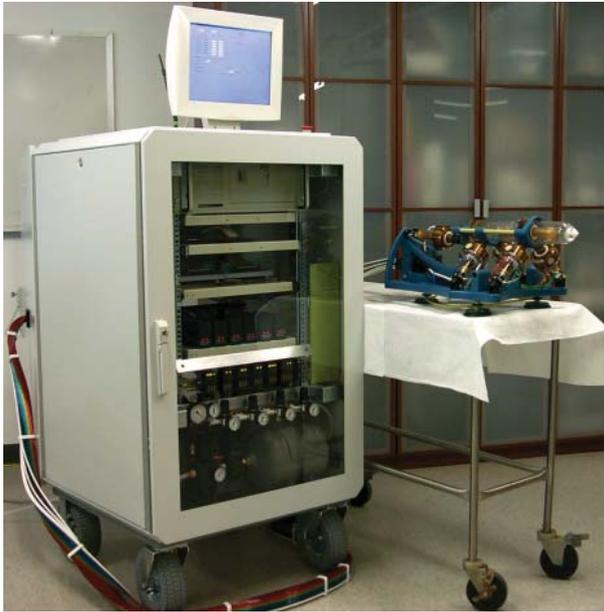
Figure 2. MR compatible fully automated brachytherapy system
