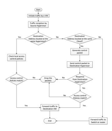
Figure 3. General mechanism flowchart.
