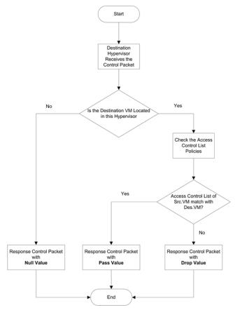
Figure 4. Destination hypervisor's tasks after control packet reception.
