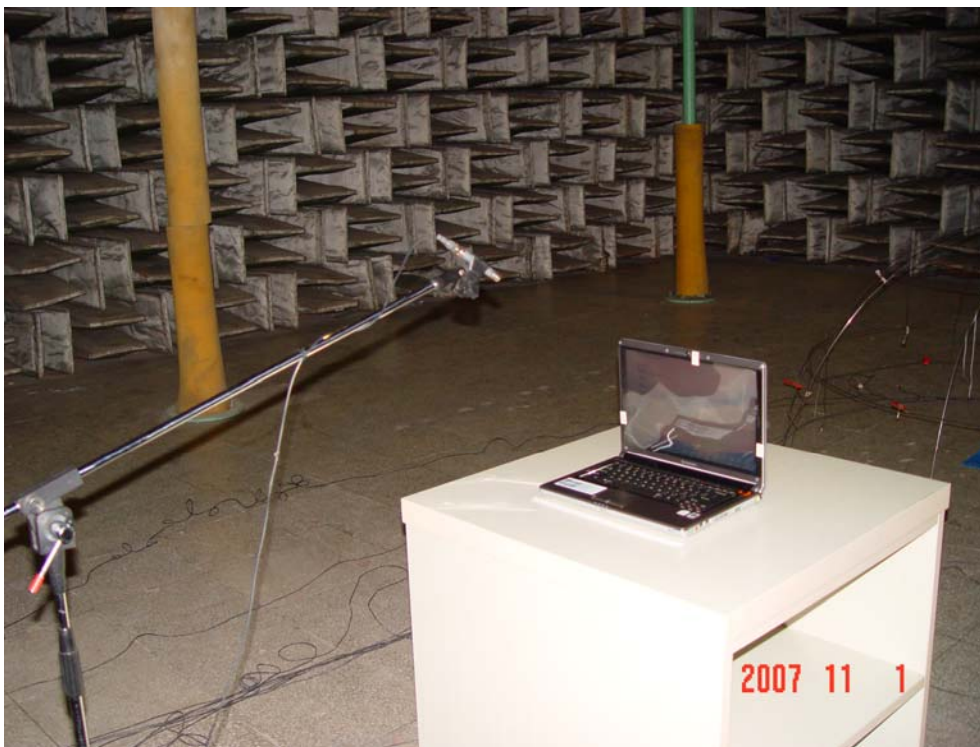
Figure 2: Actual placement of microphone, laptop and standard desk during standard desk measurement of noise radiation of a laptop.
