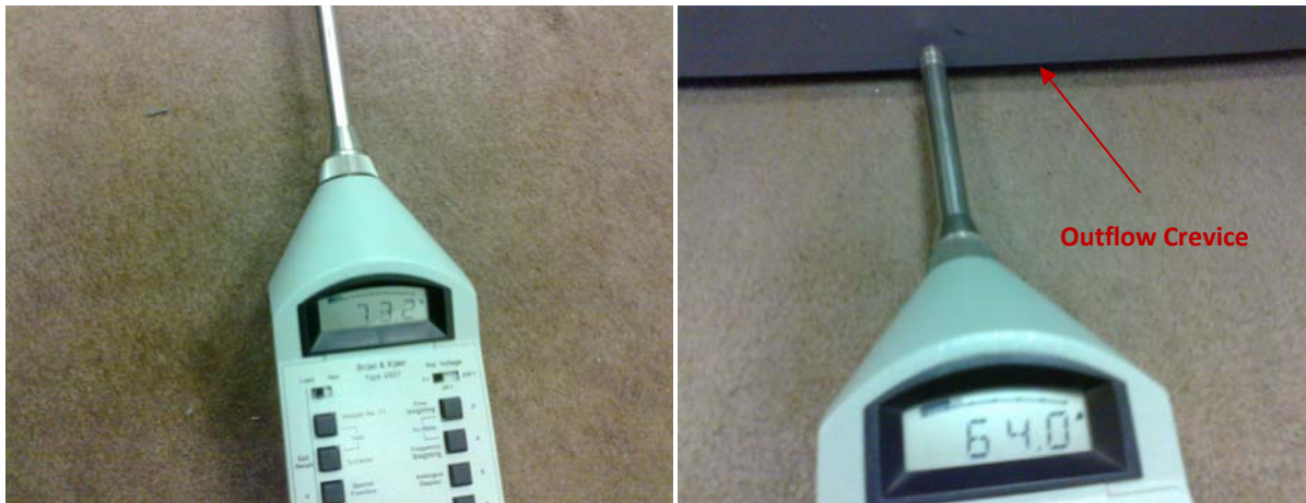
Figure 14 - Sound Power Level, before (left) and after (right) the vibration isolation.
