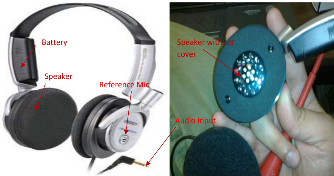
Figure 9 - Sony NC-6 Active Noise Cancellation Headphones (Left: intact and Right: with cup cover removed)
