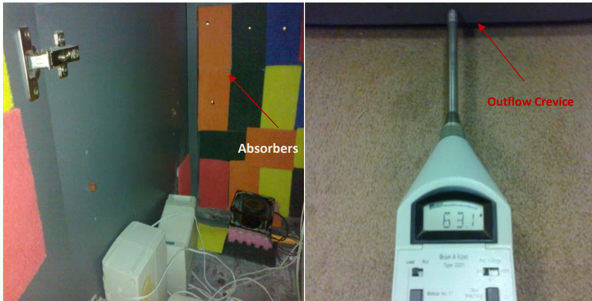
Figure 15 - Noise Absorbers (left) produced a further 1dbA reduction (right) in noise SPL
