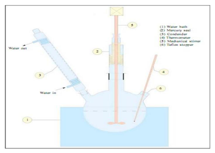
Figure 2. Esterification/Transesterification set-up.
