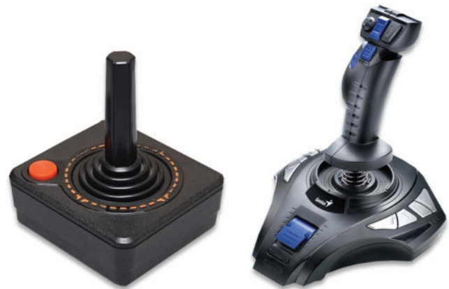
Figure 2. Left: the joystick of 1977 for the Atari 2600 game console; right: a modern joystick with multiple action buttons
