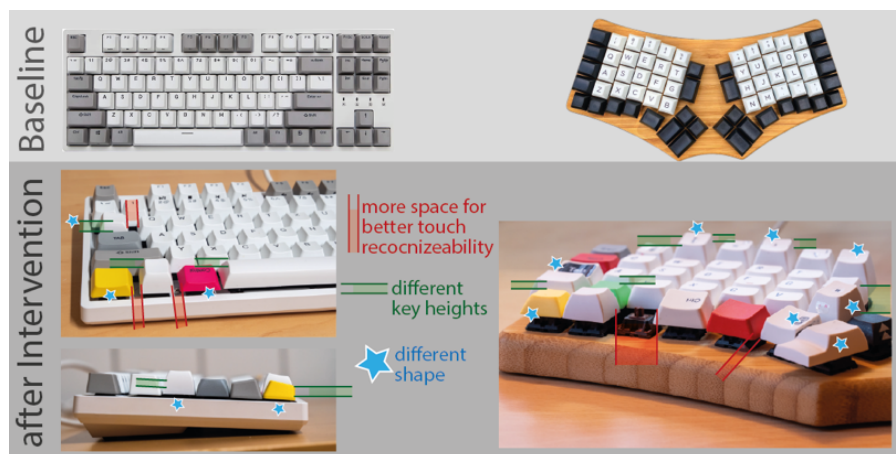
Fig. 2: Two of the keyboards with changes during intervention
