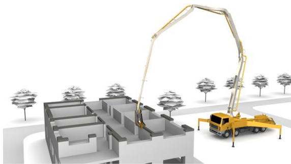
Figure 4. Schematic of CONPrint3D [13]
