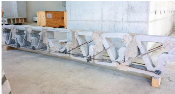
Figure 7. The first 3D printed modular reinforced concrete beam of about 3 m long [17]
