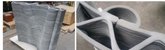
Figure 5. Multifunctional wall element [10]
