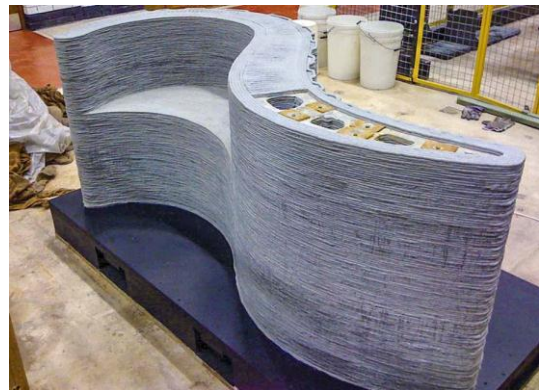
Figure 3. A full scale bench fabricated by the Concrete Printing with functional voids and post-tensioned reinforcement [12]
