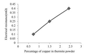
Figure 7. Changes in electrical resistance of welded specimens versus the copper content of thermite powder.
