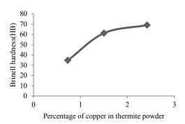
Figure 6. Hardness changes compared to the percentage of copper in the thermite powder mixture
