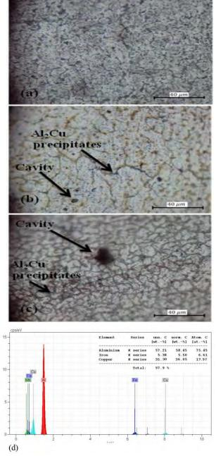
Figure 5. Cross section of specimens with (a) 0.73% (b) 1.5% (c) 2.4% of copper in thermite powder mixture and (d) EDS spectroscopy of precipitates.
