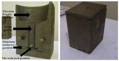
Figure 1. Graphite mould used for thermite welding of aluminum conductor.
