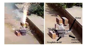
Figure 3. The graphite mould sealed before and during the test
