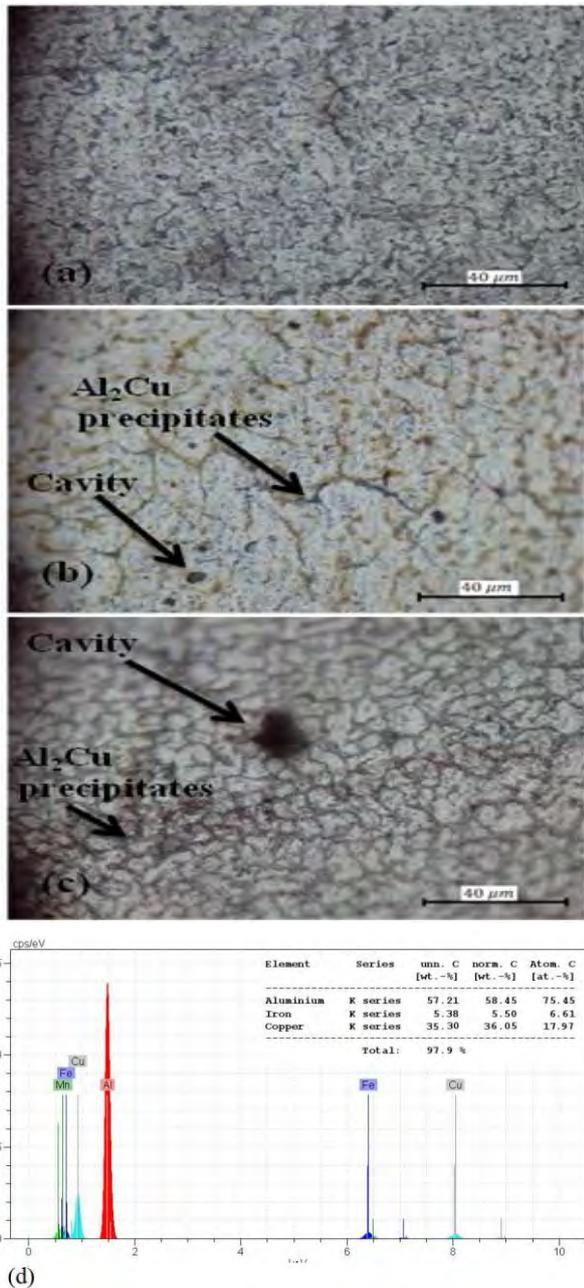
Figure 5. Cross section of specimens with (a) 0.73% (b) 1.5% (c) 2.4% of copper in thermite powder mixture and (d) EDS spectroscopy of precipitates.
