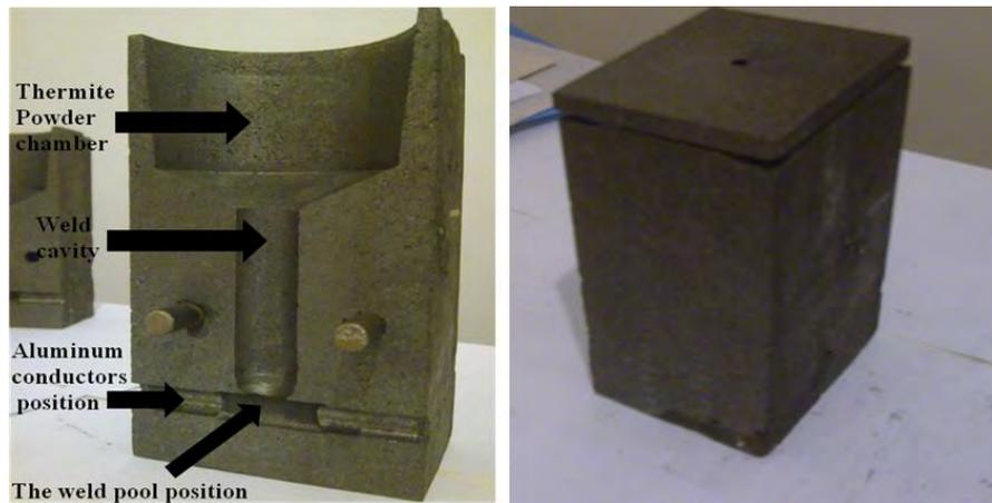
Figure 1. Graphite mould used for thermite welding of aluminum conductor.
