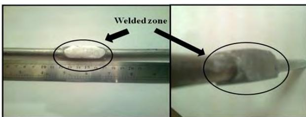
Figure 4. A sample of welded aluminum conductors
