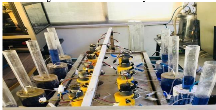
Figure 1 Semi-Automatic Methane Potential Test System (SAMPTS )
