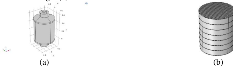
Fig. 1 (a) Model of packed bed PCM module. (b) Copper mesh added in packed bed.
