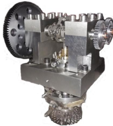
Figure 1 Rhombic drive mechanism of beta Stirling engine
