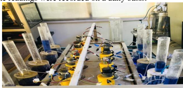
Figure 1 Semi-Automatic Methane Potential Test System (SAMPTS )
