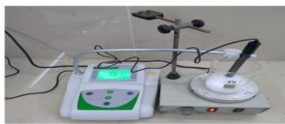
FIGURE #02 [pH Meter Electrode Placement and Showing pH 8]
