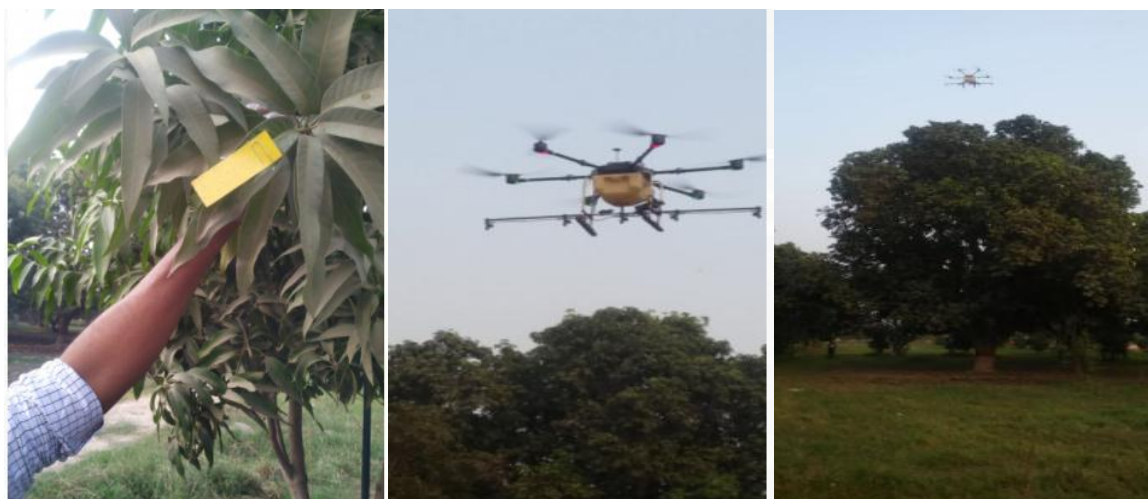
Figure 2 Water sensitive paper Sampler and UAV sprayer spraying on mango plant
