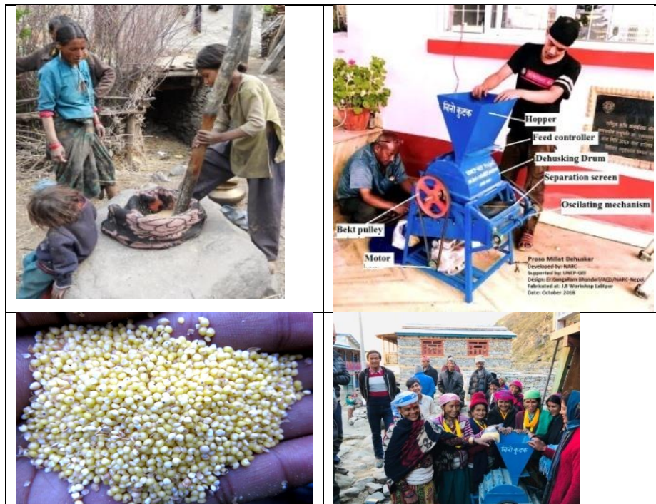
Picture 1. Dehusking by traditional method, testing at Agriculture Engineering Division, Khumaltar, dehusked grain, farmer participation during field testing in Nalla village, Humla.
