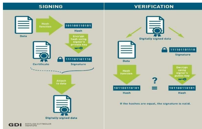
Fig. 2. Certification of digital data using blockchains [3]
