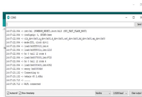
FIGURE 11. Wifi connection status displayed on Arduino IDE.
