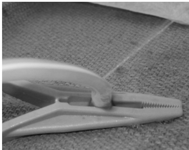
Figure 2 — Leak from a micropuncture when fluid was infused under pressure against a clamped distal end.
