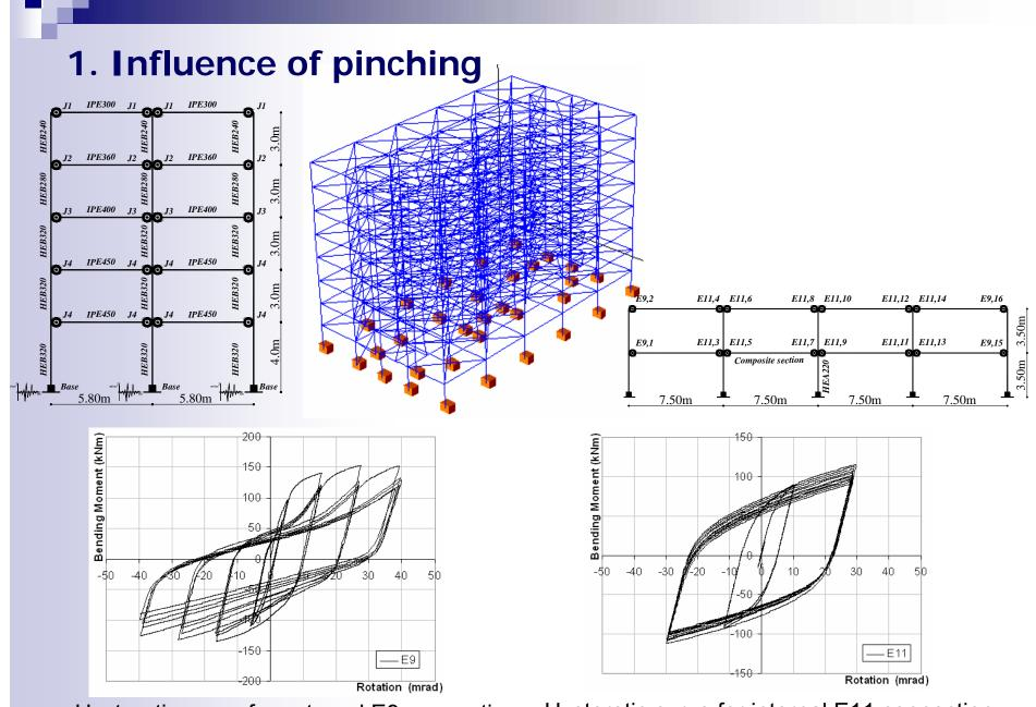
Hysteretic curve for external E9 connection Hysteretic curve for internal E11 connection
