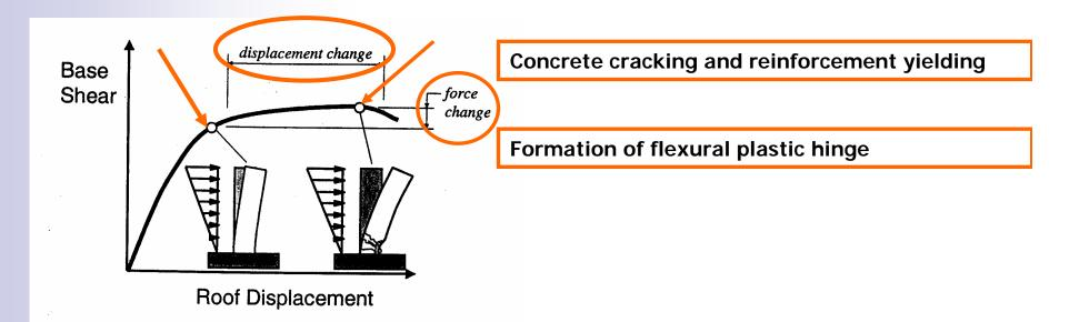
The extent of damage is related to the amount of deformation (turn to displacement) in plastic hinge
