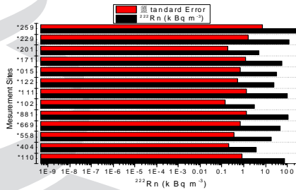
Fig. 4 ^{222}\text{Rn} concentrations vs. measurement sites. *259 representative of high concentration, while *102 representative of low concentration in NMP, the scale type \text{Log}_{10} .
