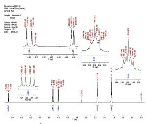
Figure 4. <sup>1</sup>H\_NMR spectrum of divinyl ester of adipic acid
