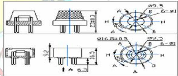
Fig 7: MQ-2 Gas Sensor Configuration
