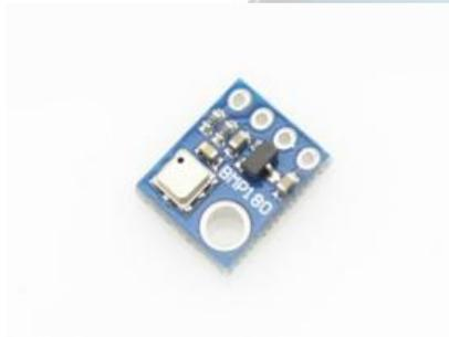
Fig5:BMP180 Pressure Sensor
