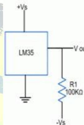
Fig4: Circuit Diagram Of LM35
