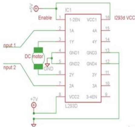
**Fig8: Circuit Diagram of Motor Driver IC**
