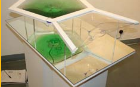
1:6 scale model showing a complete and section through an algae tank
