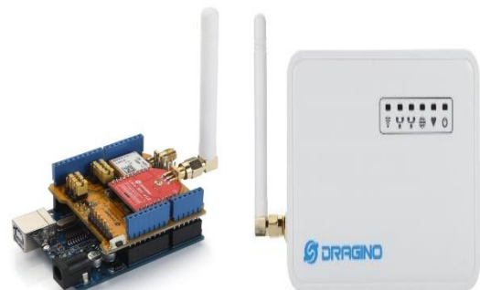
Fig. 5: LoRa Shield with Arduino UNO and Gateway
