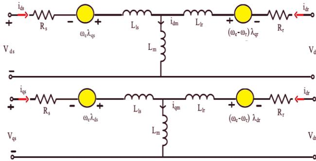
Fig. 3. "T-form" equivalent circuit for DFIG
