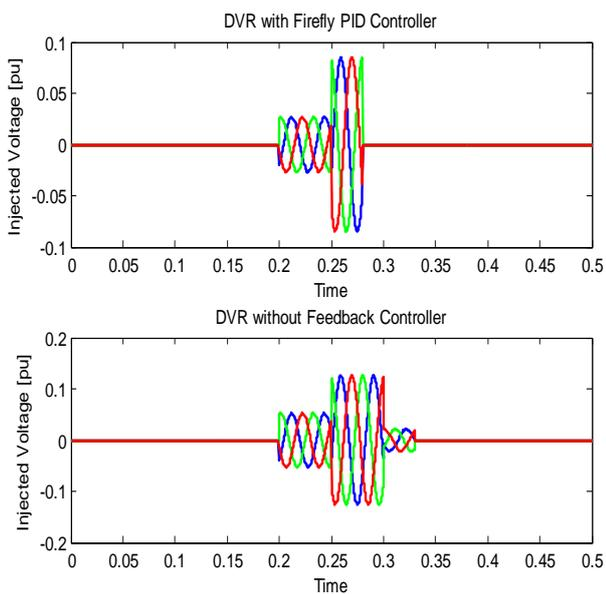
Fig. 13. Injected voltage to grid from DVR
