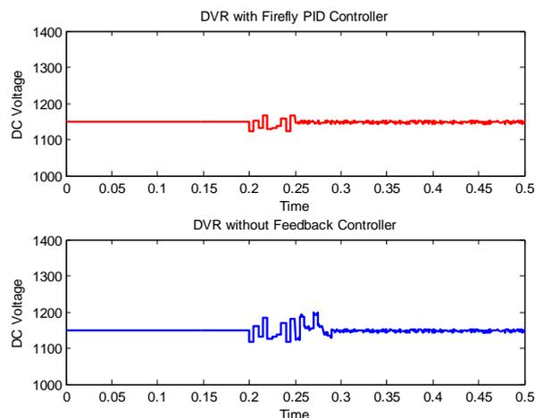
Fig. 9. DC voltage of the grid in the simulation
