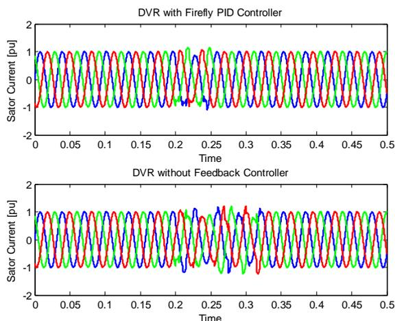
Fig. 7. Stator current in the simulation
