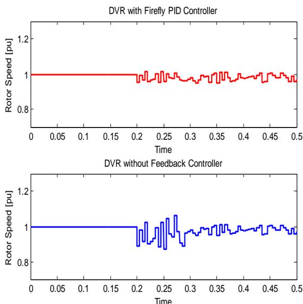
Fig. 12. Rotor speed during faults
