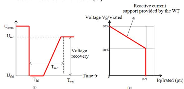
**Fig. 1.** (a) Fault Ride Through grid code ; (b) Reactive Power requirement grid code
