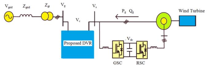
Fig. 2. Black Diagram of FRT capability in DFIG based on the proposed method
