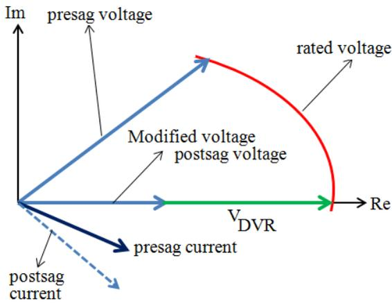
Fig. 4. Diagram of DVR based on in-phase compensation
