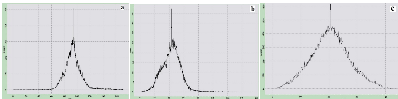
Fig. 2 Histogram of surface roughness of PP+Fe 3 O 4 nanocomposites prepared in different TTC mode: a) \beta=20^\circ/\text{min} ; b) \beta=200^\circ/\text{min} c) \beta=2000^\circ/\text{min}
