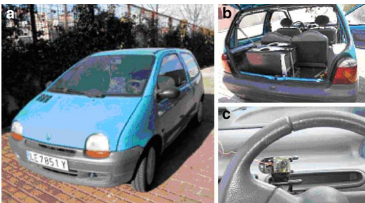
Fig. 25 a IVVI vehicle, b processing system, c driver’s camera
