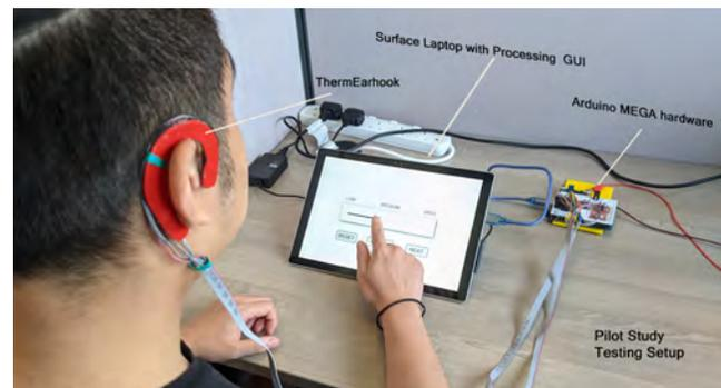
Figure 3: Testing setup with the participant wearing the ThermEarhook
