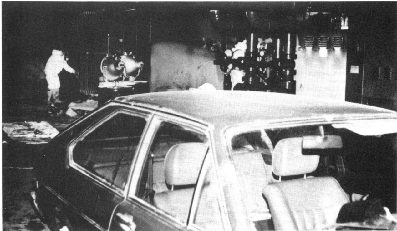
FIGURE 6. A car in the electrical room area was contaminated with PCBs and presumably other chemicals. The PCB contamination which can be visualized on top of the car could not be removed by repeated scrubbing and detergent in steam cleaning. The car was eventually removed to a toxic waste dump.
