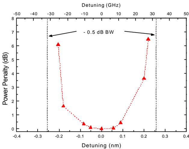
Figure 11 – Power penalty of the removed channel as functions of the channel spacing.
