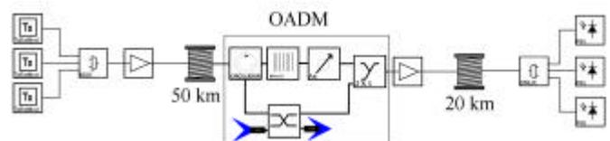
Figure 1 – Scheme of the OADM and experimental transmission DWDM network.
