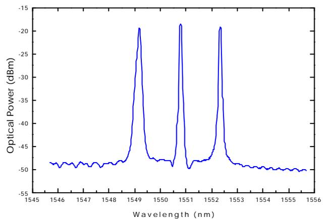
Figure 6 – Output signal with an added channel.
