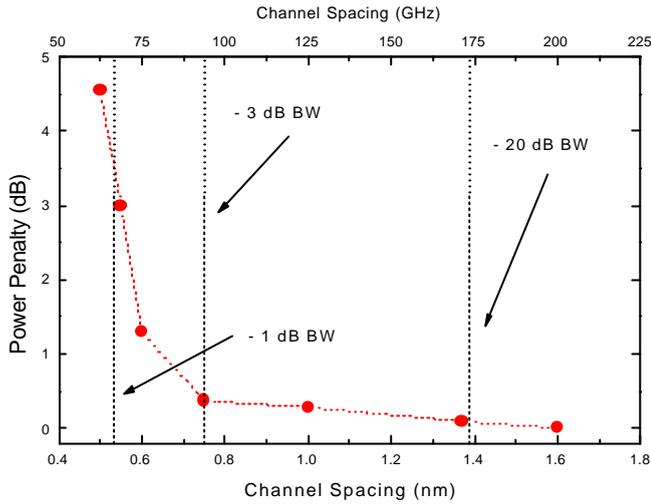
Figure 10 – Power penalty of the removed channel as functions of the channel spacing.
