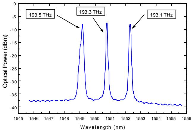
Figure 3 – Input signal at the OADM
