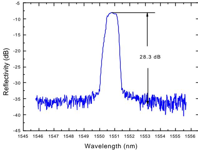
Figure 2 – Reflection spectra of the FBG.
