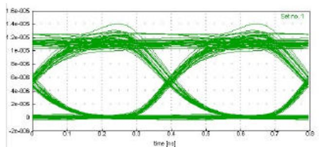
Figure 13 – Simulated eye diagram for the dropped channel.
