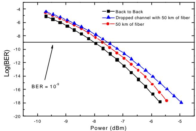
Figure 12 – Simulated BER performance for the dropped channel.
