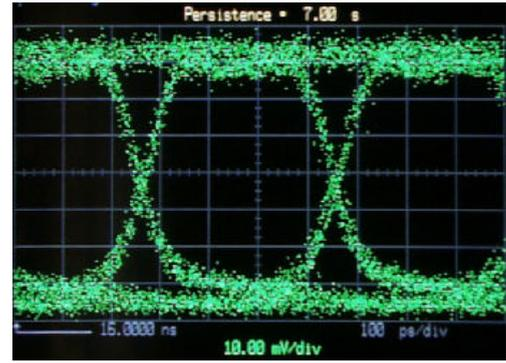
Figure 8 – Eye diagram for the dropped channel.
