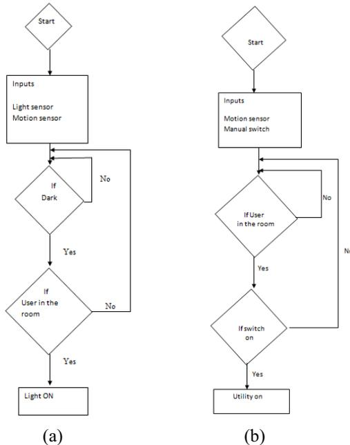
Figure 2. Overview of the (a) lighting system, (b) utilities system
