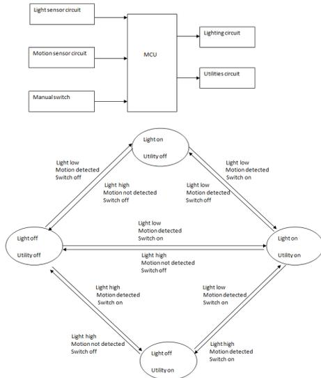
Figure 1. System overview and state diagram
