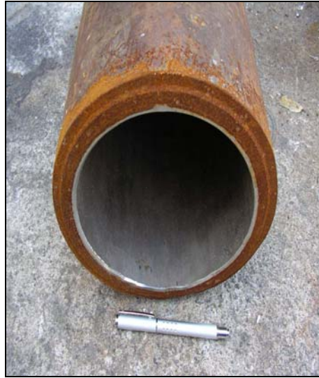
Figure 5 – Clad Pipe (3mm Inconel 625 + X65 carbon steel)
