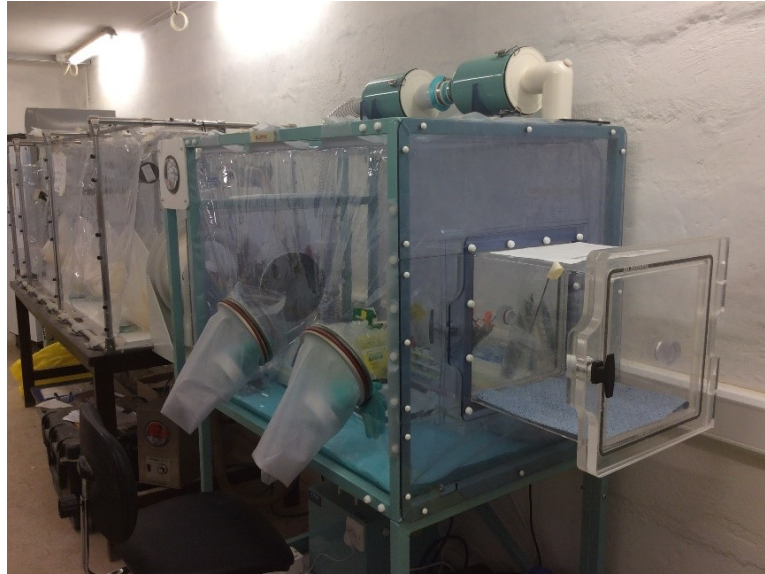
Figure 1. The real isolator. The pass box is shown to the right, and the sleeved gloves are shown.
