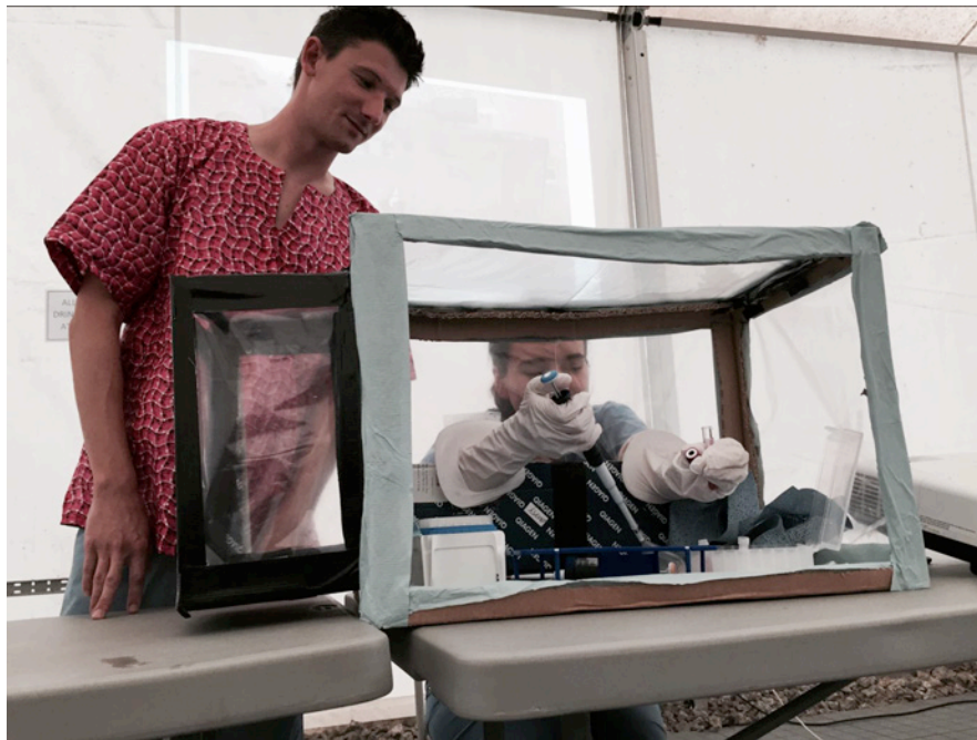
Figure 4. The mock isolator used in Sierra Leone for teaching /demonstrating purposes. The pass box is shown to the left.
