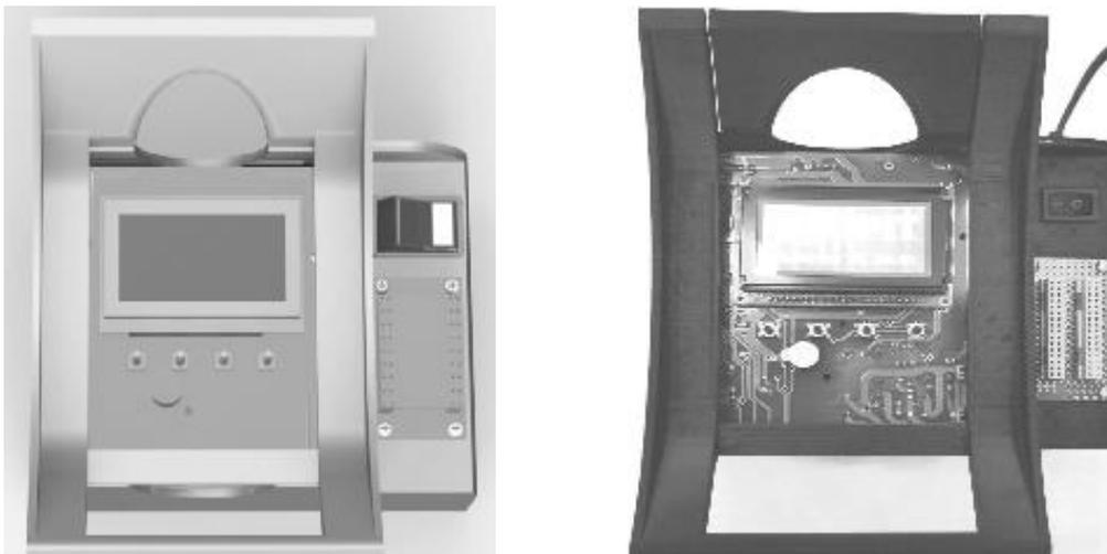
Fig. 02 Visualisation of a quality control device and its 3D printed version.
