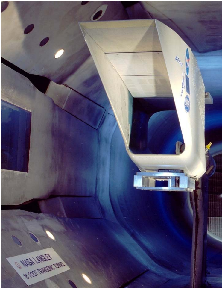
Fig. 1.21. The SAMPSON F-15 inlet cowl as installed in the NASA Langley Transonic Wind Tunnel [82, 89].
