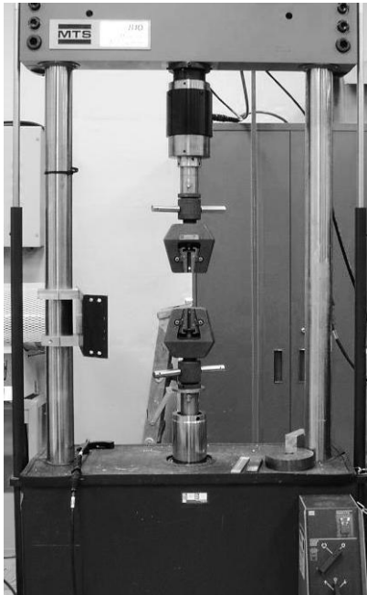
(a) MTS 810 servohydraulic loading frame.
