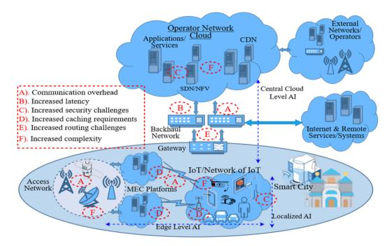
Figure 2. Network Architecture of 5G using Machine Learning [5]
