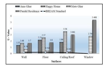
Figure 12. Comparative Study of Calculation of U-Values of different surfaces of the Case Studied buildings
