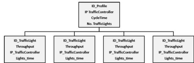
Fig. 2. Global structure of the traffic control profile.
