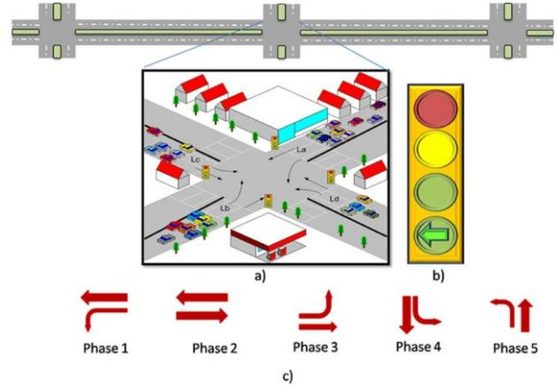
Fig. 1. Model description. Our approach is based on a multi-intersection scenario with four traffic-lights. a) Model of an isolate intersection. b) traffic-light used in our model. c) phase model.
