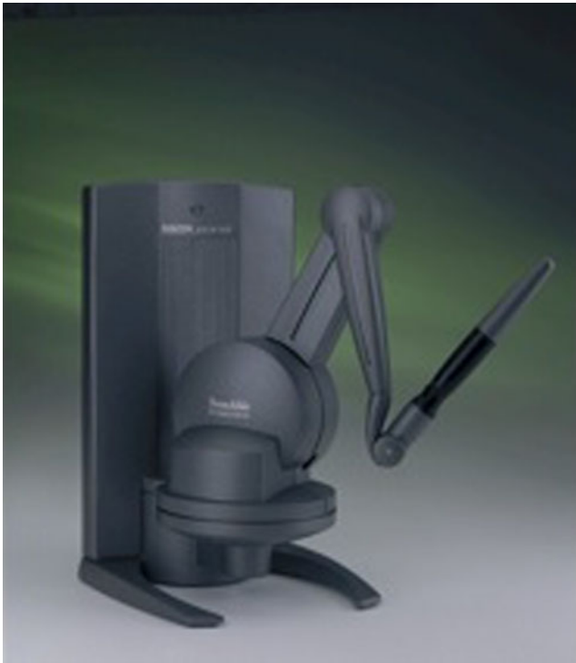
Fig. 8 A haptic device (SensAble Technologies, Woburn, Massachusetts) for use in the digital dental laboratory; intuitive manipulation of the on-screen object with proprioceptive feedback
