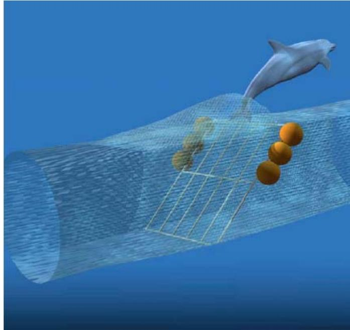
Figure 2. Diagram of the dolphin exclusion device tested by Northridge 2003a,b, and Northridge et al. 2003, drawn approximately to scale (dolphin = 2m in length). (Figure from Northridge 2003b)
