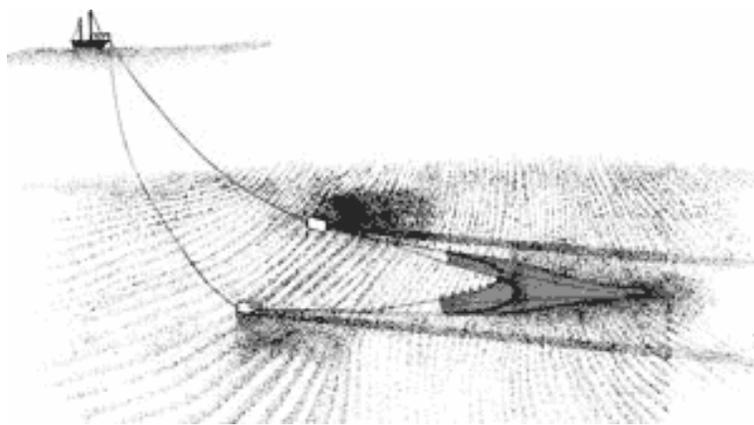
Figure 1. Diagram of a bottom trawl net. A mid-water trawl would be configured similarly, but it would be towed at mid-water depths while a pair trawl net is usually larger and towed by two vessels. (Diagram by Dr. Joe DeAlteris, University of Rhode Island)
