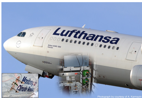
Fig. 2. IAGOS-CORE installation position aboard the Lufthansa A340-300 ‘Viersen’ (photograph by courtesy of A. Karmazin); the inset shows details of the IAGOS Inlet Plate, which carries the inlet probes for trace gas sampling (photograph by courtesy of Lufthansa).
