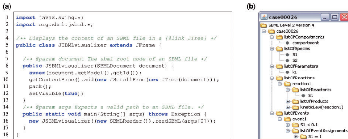
Fig. 1. (a) The SBML parser in JSBML understands the hierarchical data structure of SBML; (b) Example for SBML test case 26. Using JSBML for reading and visualizing an SBML file. The type SBase extends the Java interfaces Serializable for saving JSBML objects in binary form or sending them over a network connection, Cloneable for creating deep object copies and TreeNode . The last interface allows callers to apply any recursive operation, such as using JTree for display [see (b) for an example].
