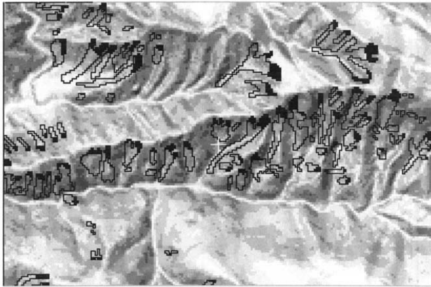
Figure 1. Scars of the past landslides induced by the 1994 Northridge Earthquake in California, U.S.A. The areas shown in black within the landslide bodies were considered as scarps of the landslides.
