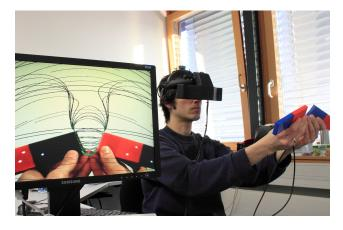
Fig. 4. AR setup using a video see-through HMD with included tracking and real magnets as interaction device. The separate monitor displays the image generated for the user's left eye.
