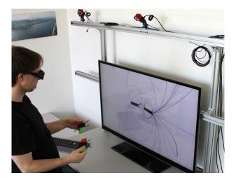
Fig. 5. VR setup using an active stereo LCD-TV, optical tracking and real magnets with tracking markers as interaction devices.
