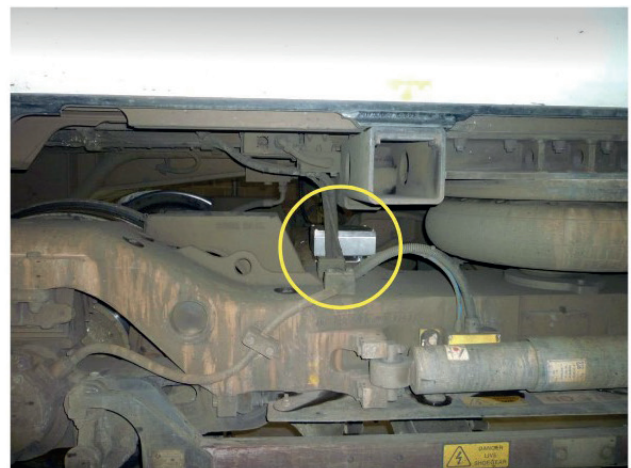
Fig. 2 IMU positioning on the bogie (Yeo, 2017:p.48)
