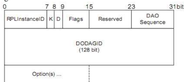
Fig 5: DAO message structure
