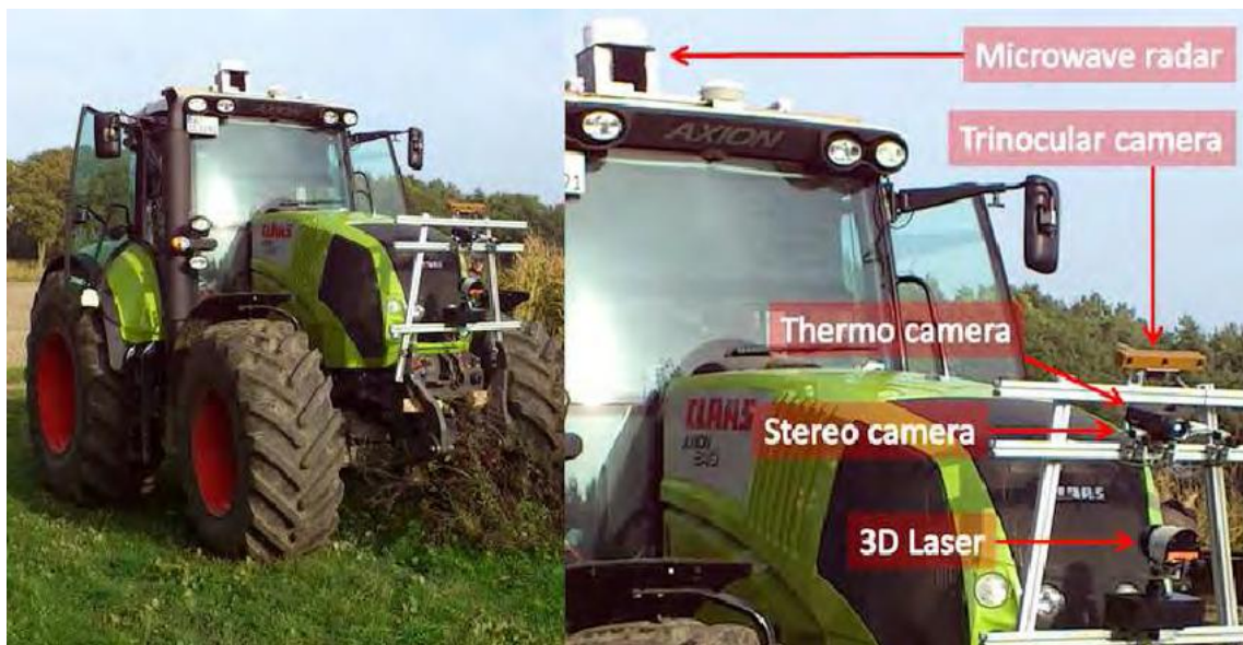
Fig. 4(A) Proposed Design2 of Digital Camera System Fitted on Tractor used for image processing techniques employing IOT, ML & AI Tools using MATLAB Software as Platforms for plant disease detection
