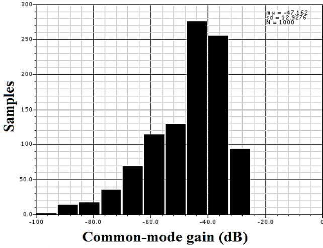
Fig.8. Monte Carlo simulation of the common-mode gain of the proposed OTA for 1000 samples
