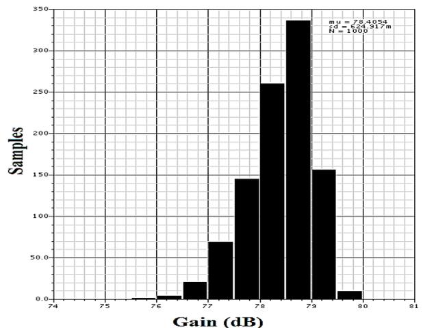
Fig.7. Monte Carlo simulation of the DC gain of the proposed OTA for 1000 samples
