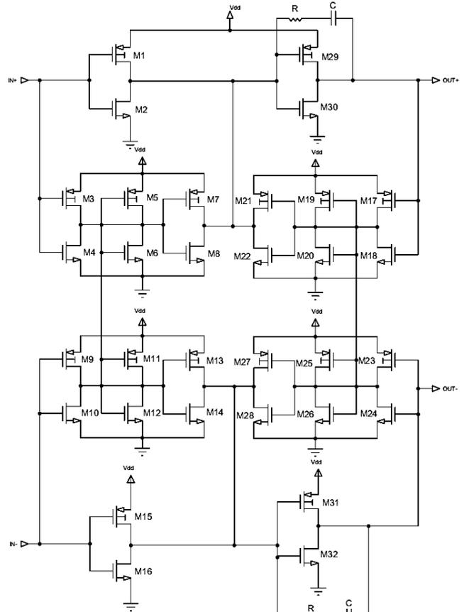
Fig.2. Schematic of the proposed two-stage OTA
