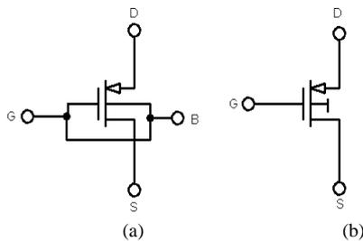
Fig.1. DTMOS technique (a) equivalent circuit, (b) symbol
