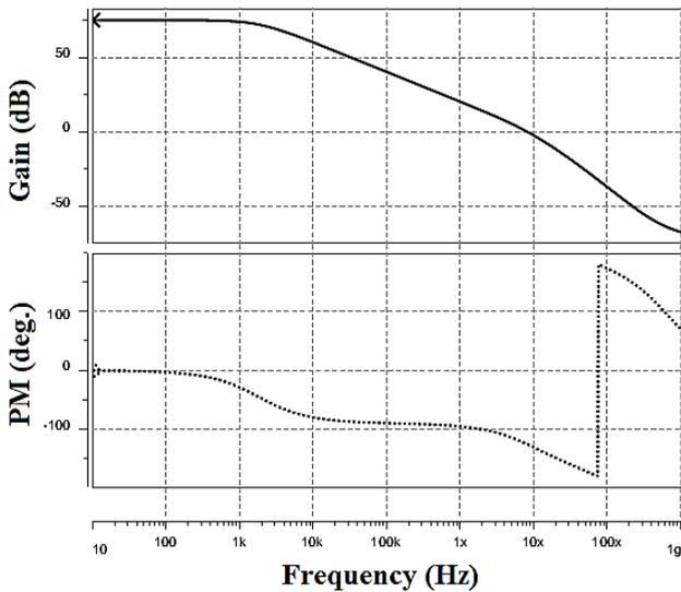
Fig.3. Open loop gain and phase margin of the proposed OTA
