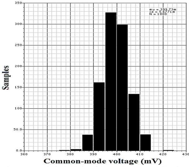
Fig.9. Monte Carlo simulation of the output common-mode voltage of the proposed OTA for 1000 samples
