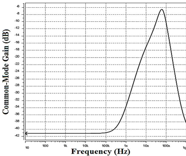
Fig.4. Frequency response of the common-mode gain of the proposed OTA
