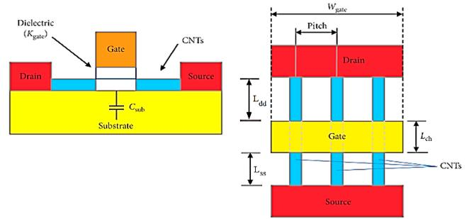
Fig. 1. Structure of a C-CNTFET [8]
