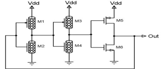
Fig. 5. Proposed design 3 for a 3-stage ring oscillator
