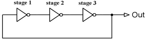
Fig. 2. Block diagram of 3-stage ring oscillator
