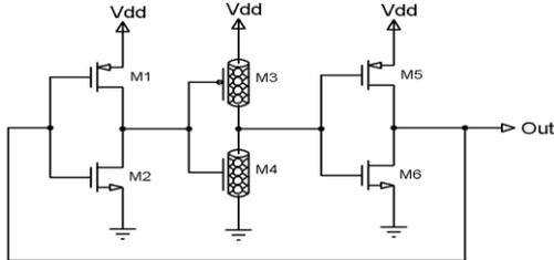
Fig. 3. Proposed design 1 for a 3-stage ring oscillator
