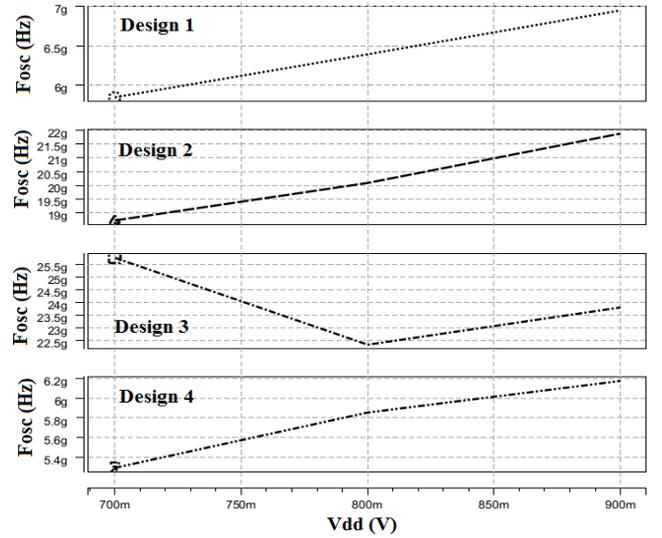
Fig. 7. Oscillation frequency variation in terms of supply voltage change for different structures of the proposed 3-stage ring oscillator
