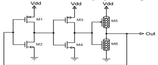
Fig. 6. Proposed design 4 for a 3-stage ring oscillator
