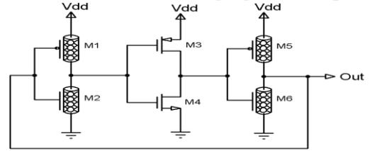
Fig. 4. Proposed design 2 for a 3-stage ring oscillator
